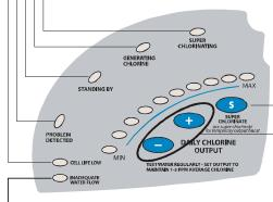
Illuminates when there is no flow or low flow through the Cell. The pool filter pump could be in its "off" cycle. If this is not the case, refer to the Troubleshooting section in this manual.
