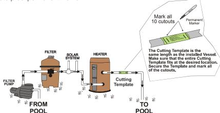
Remove the Template, cut the pipe and install the Nut Assemblies as shown below. Use the included 2" Nut Assembly for 2" pipe and  $1\frac{1}{2}$ " Nut Assembly for  $1\frac{1}{2}$ " pipe. Place Nut Assembly on each side of the cut pipe (threads face in). Be sure to place the Nut, Compression Ring and Collar on the pipe as shown in the diagram.
