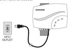
After being powered on for the first time, the Salt & Swim will run a diagnostic routine which can take up to 30 seconds. During this time, various LEDs will turn on and off. When finished, the Salt & Swim will display a *blinking* INAD-EQUATE WATER FLOW LED and a *solid* STANDING BY LED. Keep the Salt & Swim powered for the remainder of this procedure and go to Step 3.
